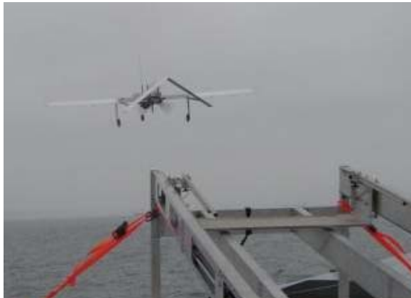
Figure 4. Manta UAV being catapult launched from the Stiletto Experimental Hull Vessel.
