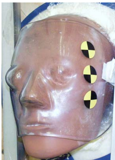
Figure 10: Custom face shield fitted to a Hybrid III 50th percentile dummy.
