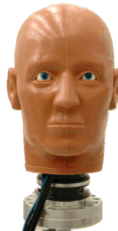
Figure 1: The FOCUS headform is designed to predict the risk of eye and facial injuries.
