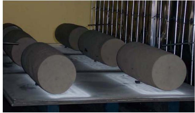
Figure 2. PM Ti-6Al-4V extrusion billets shown in the vacuum sintering furnace after densification.
