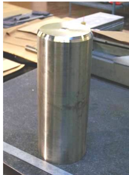
Figure 3. A 14 cm dia. x 35 cm long CIP/sintered/ground preform input billet prepared for rotary forge conversion into 2.22 cm dia x 3.66 - 4.57 m length Ti-6Al-4V rod.
