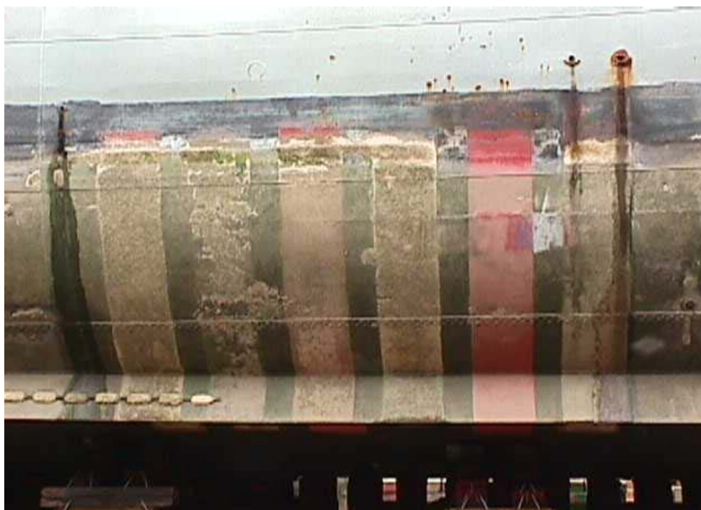
Figure 18: Starboard side strips on HMAS BRISBANE, March 1999. Ecoloflex strip is second from right.
