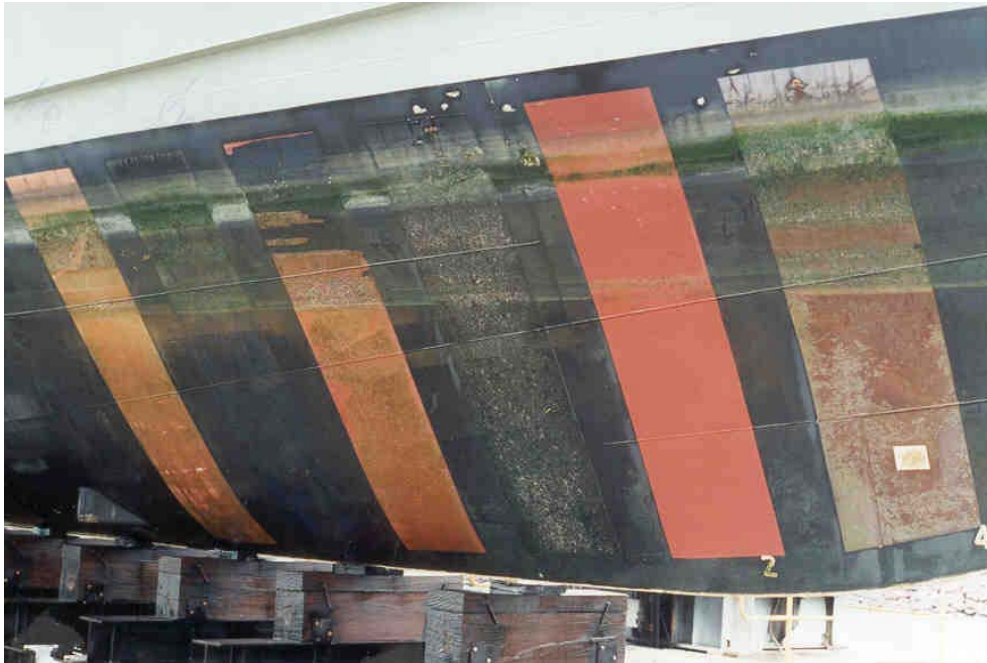
Figure 11: Starboard side strips on HMAS BENDIGO, February 1995. Ecoloflex strip is second from right.
