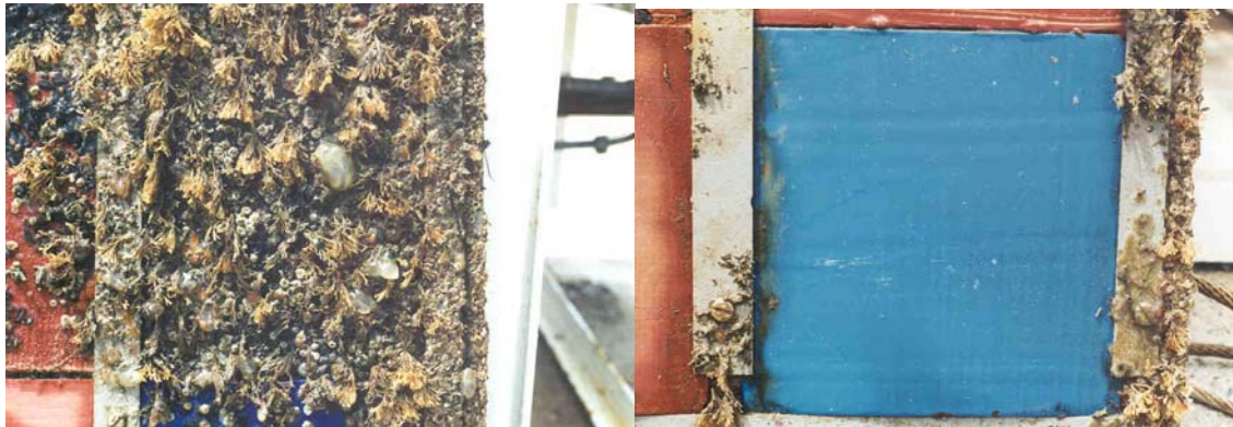
Figure 8: Ecoloflex panel (right) and non-toxic control (left) after static immersion during 1996/1997 rotor trial
