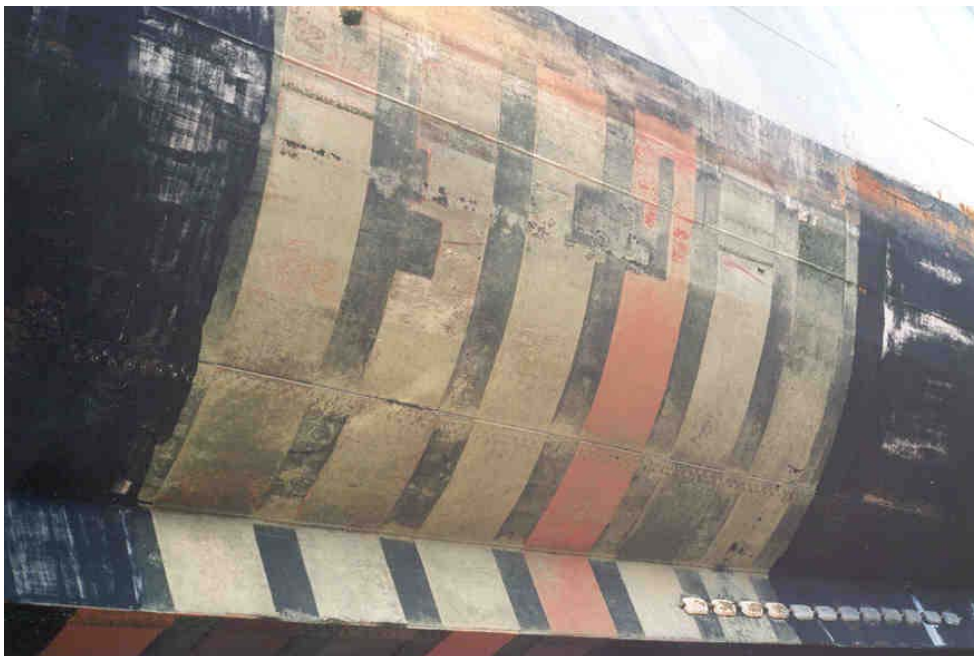
Figure 17: Port side strips on HMAS BRISBANE, May 1996. Ecoloflex strip is third from right.
