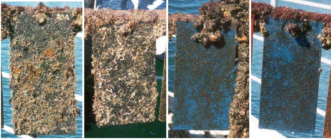
Figure 1: Test panels on Williamstown raft, 23 March 2000: left, control panels after 43 days immersion; right, Ecoloflex panels after 39 months (first immersed 23 Dec 1996)
