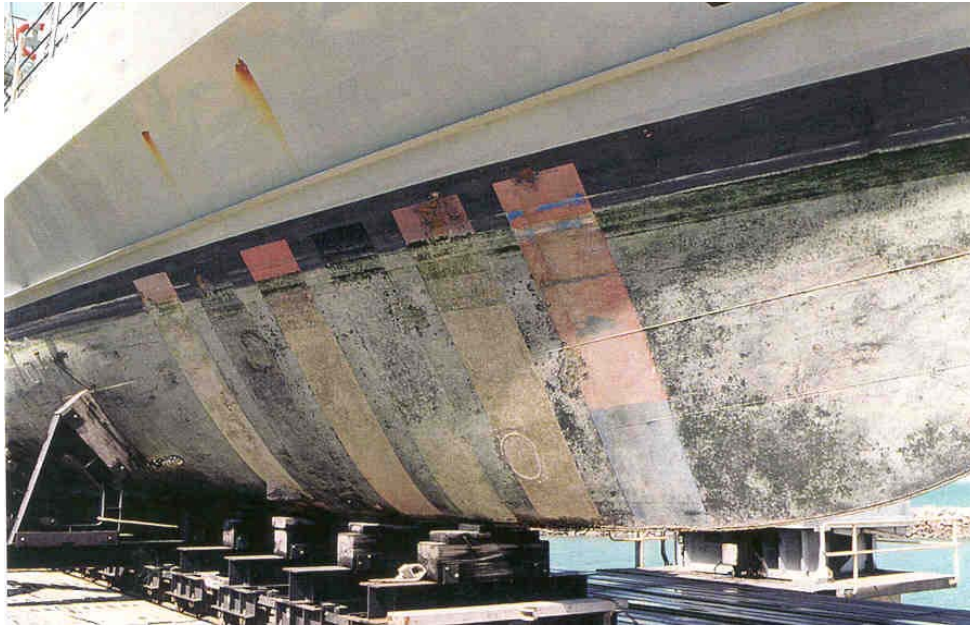
Figure 15: Starboard side strips on HMAS BUNBURY, May 1998. Ecoloflex strip is first from right.
