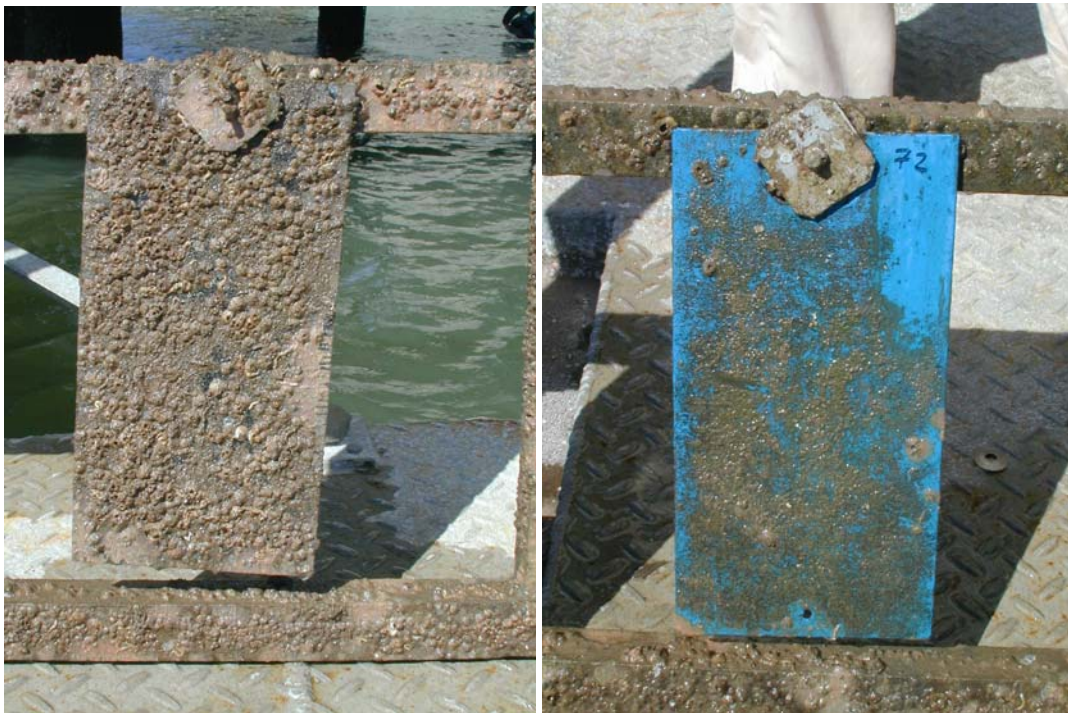
Figure 2: Test panels on Cairns raft, 12 May 2000: left, control panel after approximately 3 months immersion; right, Ecoloflex panel after 33 months (first immersed 14 August 1997)
