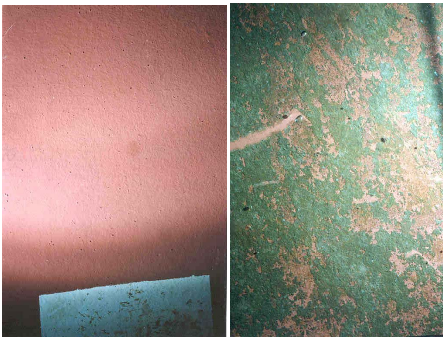
Figure 10: Underwater photographs of Ecoloflex strip on HMAS BENDIGO in January 1995 (left) and October 1997 (right) showing only slime
