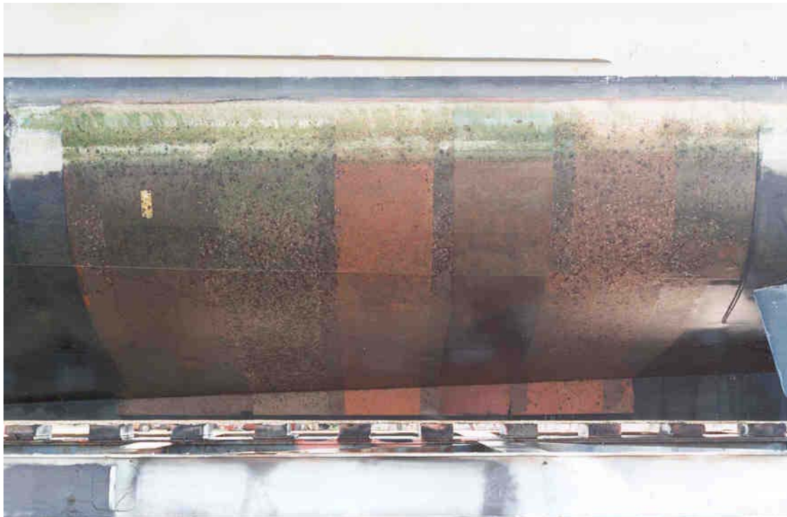
Figure 9: Port side midships test strips on HMAS TOWNSVILLE at completion of trial after 31 months
