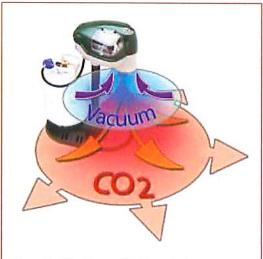
Figure 3. The Mosquito Magnet uses propane to produce  $CO_2$  and heat to attract insect vectors which are caught in the vacuum and deposited in the collection bag.
