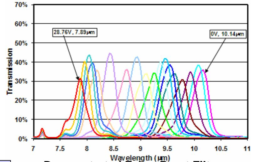
Demonstrated Fabry Perot Filters Tunable from 8 – 10 μm
