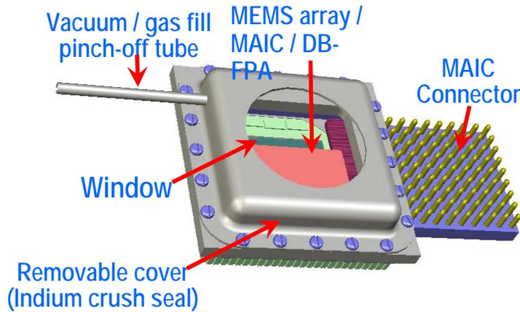
Prototype Integrated Tunable FPA Planned in FY 07
