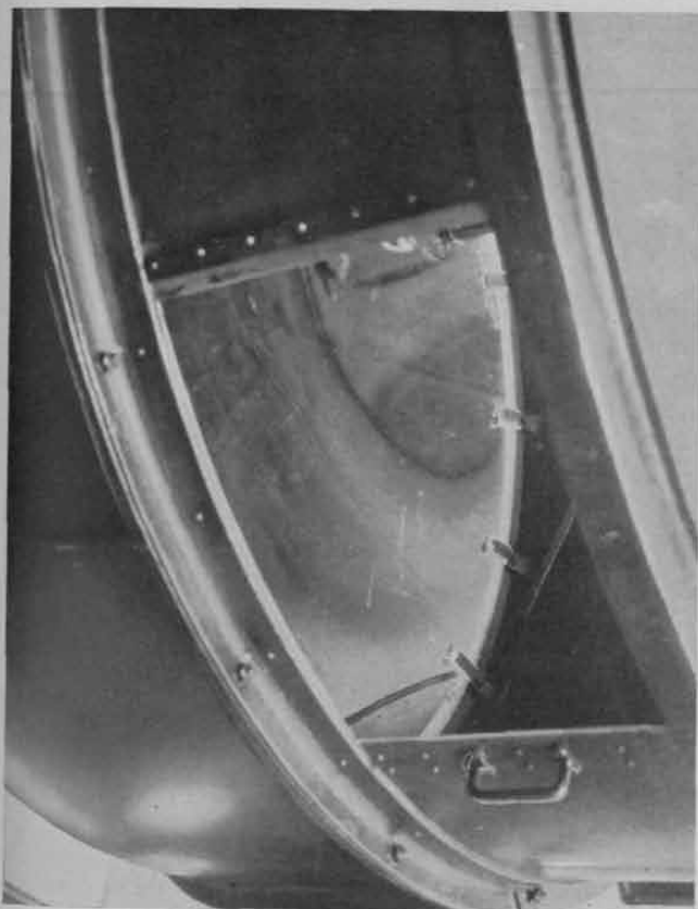
Fig. 5. Showing Clamping of Metal Mirror.
