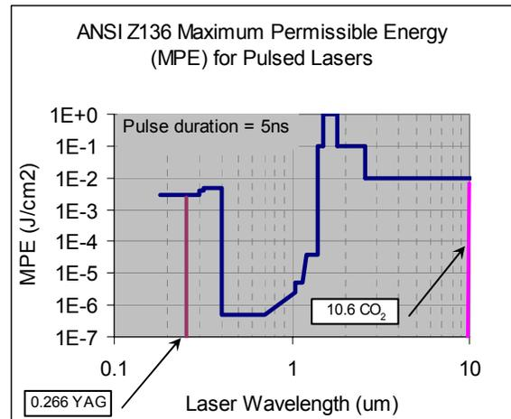
Figure 3. ANSI Z136 MPE for pulsed lasers. The TREDs-2 system wavelengths are identified.
