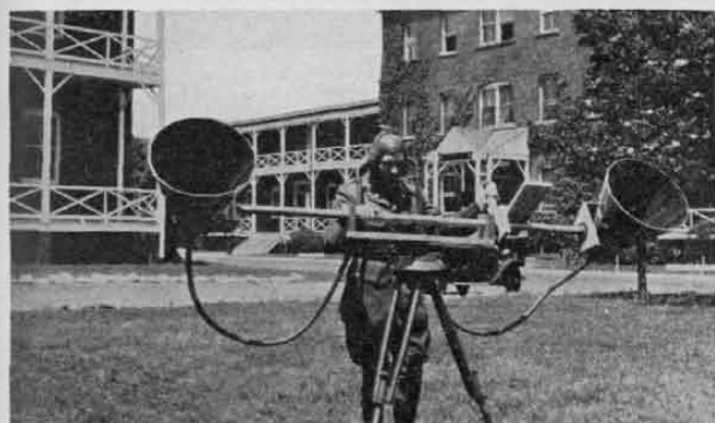
First Model of the Miniature Sound Locator.
