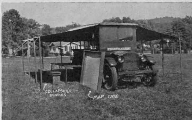
A command post truck developed by the National Guard of Pennsylvania. Walls are also provided which permit the whole outfit to be inclosed in canvas.
