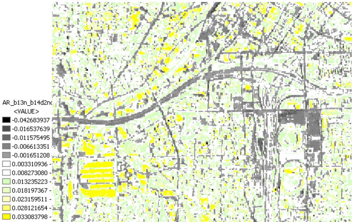
Figure 4. NDTI image based on Bands 13 and 14. The categories are 1/2 standard deviation intervals.
