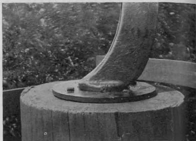
Socket and shank of machine-gun yoke.
