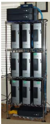
Fig. 8. The HERD-0 PC cluster assembled at SEA LLC for physical modeling work. Each of the nine nodes has a dual core Athlon 64 processor and 3 GB of RAM. The nine PCs are connected by a private Gigabit Ethernet network and are powered by uninterruptible power supplies. HERD-0 exceeded 56 Gflops/s.
