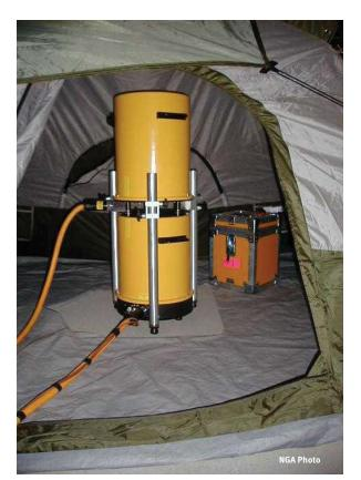
An absolute gravity meter weathers the elements during a gravity survey.
