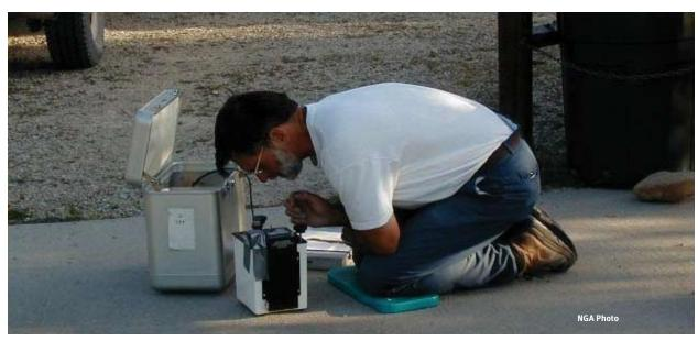
A geodetic surveyor records a measurement from a relative gravity meter.
