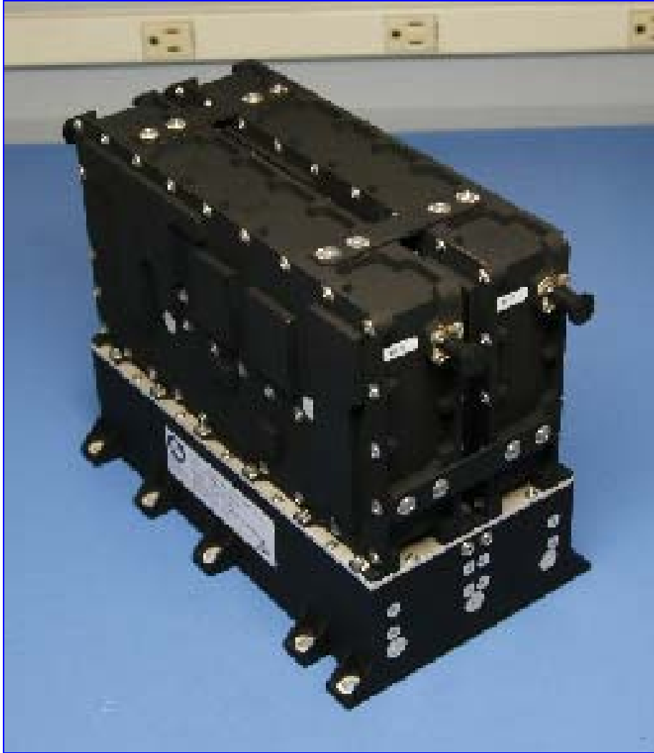
Figure 11. Dual redundant tunable frequency generators.
