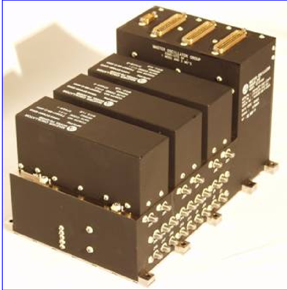
Figure 2. Triply redundant highly stable OCXO.
