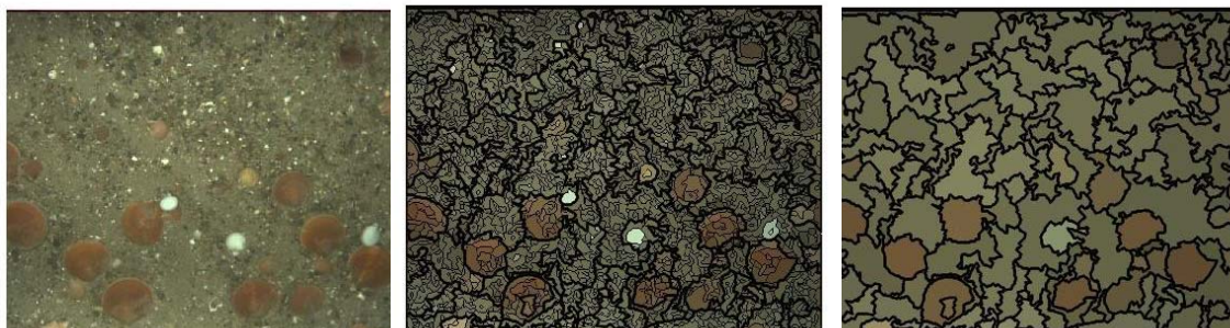
Figure 8. Segmentation of image taken in Closed Area II, HAPC of nine scallops on a sandy bottom. Raw raster image (left), fully segmented vector image (center), vector image where polygons have been aggregated based on similar color and texture features. Note that the scallops have been successfully segmented.
