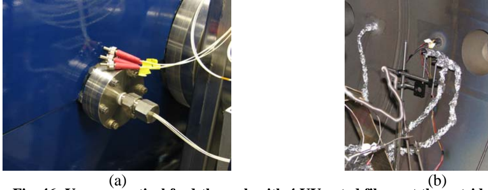
Fig. 46: Vacuum optical feed-through with 4 UV-rated fibers at the outside, and (right pane) – four 3m optical fibers shielded by foil inside the vacuum tank. Two of the fibers are attached to the mini-focusing lenses (collimators) mounted at the adjustable mechanical arms for accurate light collection
