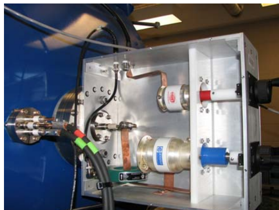
Fig. 42: Re-designed matching network box mounted to the 8-inch window vacuum port next to new high-I feedthrough. New 2.75" RF- vacuum feedthrough is attached to the window flange together with the box to eliminate leaks
