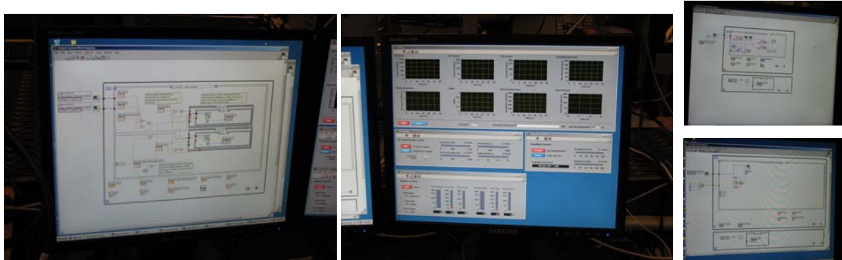
Fig. 52: center – mHTX control panel allowing real-time correction of experimental parameters, left & right sides – diagrams of the different sub-systems reflecting their status.
