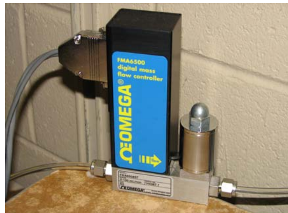
Fig. 49: 0-100scm gas flow controller is insulated from the electrical ground to eliminate RF-interference
