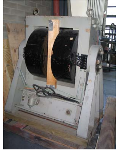
Figure 5: Existing 2-magnet MRI system by Varian was too bulky
