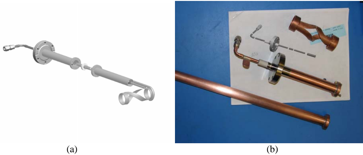
Fig. 41: (a) - CAD rendering of RF-delivery network, and (b) – machined pieces
