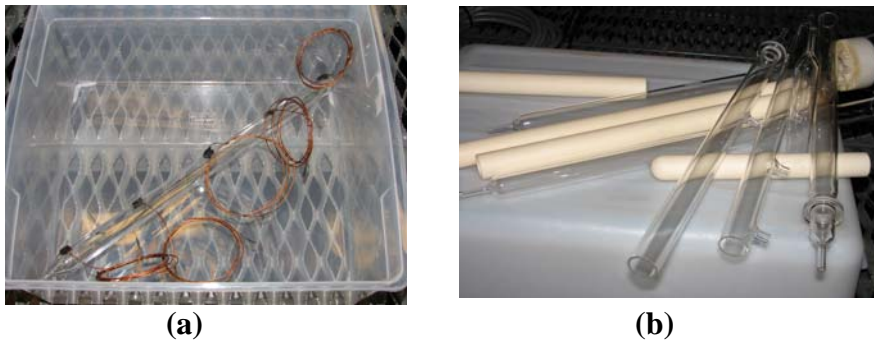
Fig. 47: (a) - standard 40-cm 2cm ID quartz tube with 5 thermocouples attached using high-conductive high-T (~600C) epoxy, (b) – various non-standard quartz and non-transparent alumina tubes were built for different mHTX experiments
