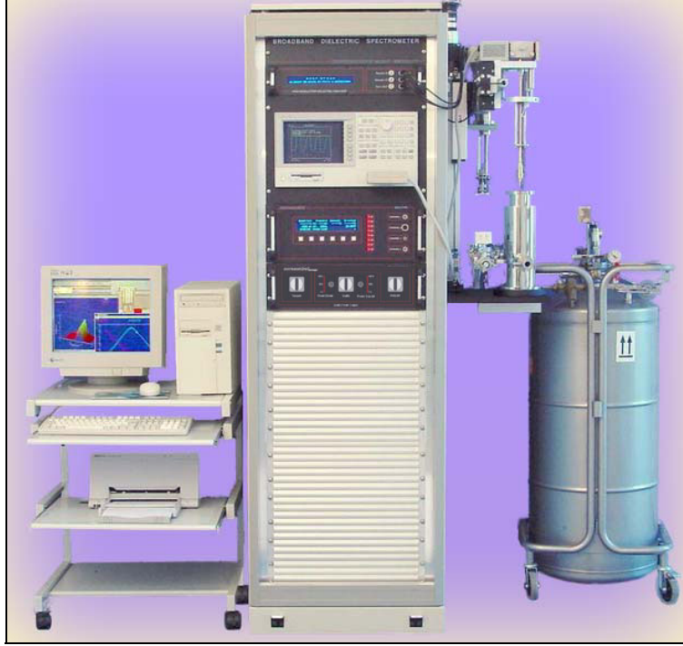
Figure 6. Broadband dielectric spectrometer by Novocontrol.
