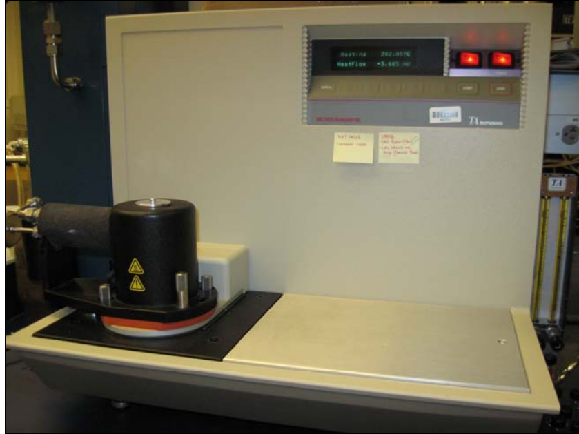
Figure 1. Differential scanning calorimeter by TA Instruments.
