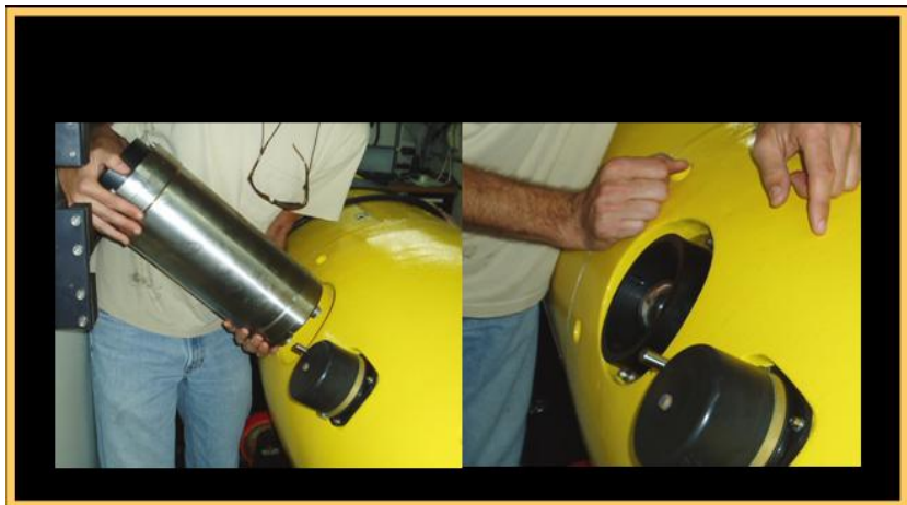
Fig. 2 The interchangeability of the electronic still camera and the sub-bottom profiler.
