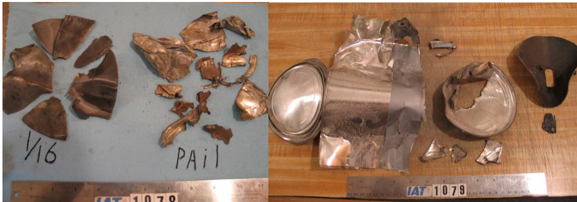
Figure 6.2. Recovered bucket parts: SCR 1078, V=981 m/s (at left) and SCR 1079, V=821 m/s.
