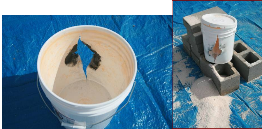
Figure 7.4. Results from Shot FT 6, striking a 5-gallon plastic bucket filled with ANFO.
