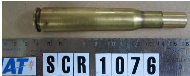
Figure 5.1. Projectile 1, a brass case filled with APEX, shown here crimped to 0.50 case.
