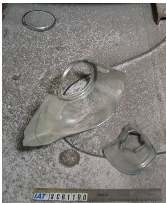
Figure 6.6. Bucket after test from SCR 1100.
