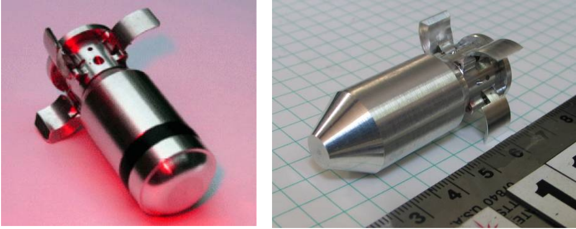
Figure 5.4. Fin-stabilized 12-gauge projectile from Special Cartridge Company shown in photograph on left and projectile 3 shown on right.
