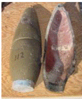
Figure 1.1. 81 mm mortar after deflagration caused by impact of a thermite-containing projectile.
