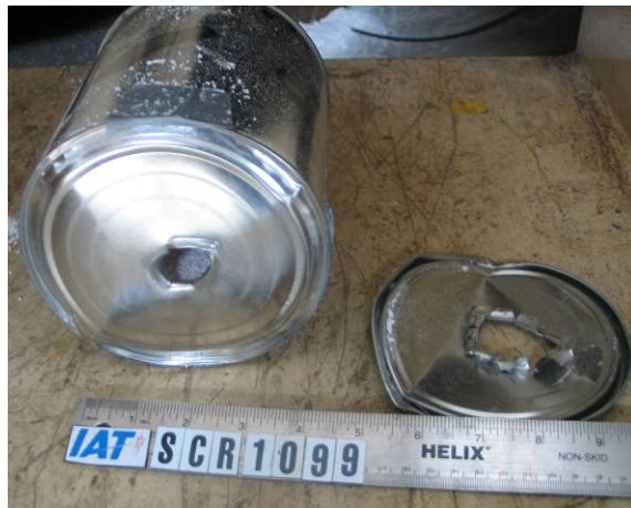
Figure 6.4. Recovered bucket from 0.50-caliber ball test (SCR 1099).
