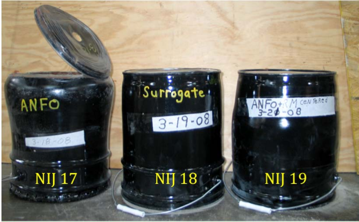
Figure 4.4. Results of tests 17–19. In test 17, APEX placed in the base plate ignited the ANFO, which blew the base open as shown. In test 18, the bucket was filled with inert material. There was insufficient overpressure from the APEX to remove the lid, and the bucket was undeformed. In test 19, the APEX and ANFO were in the center of the bucket, instead of against the base plate. Overpressure bulged the midsection of the bucket, although the bottom plate was not blown off.
