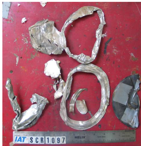
Figure 6.3. Recovered bucket and cover plate pieces from SCR 1097.
