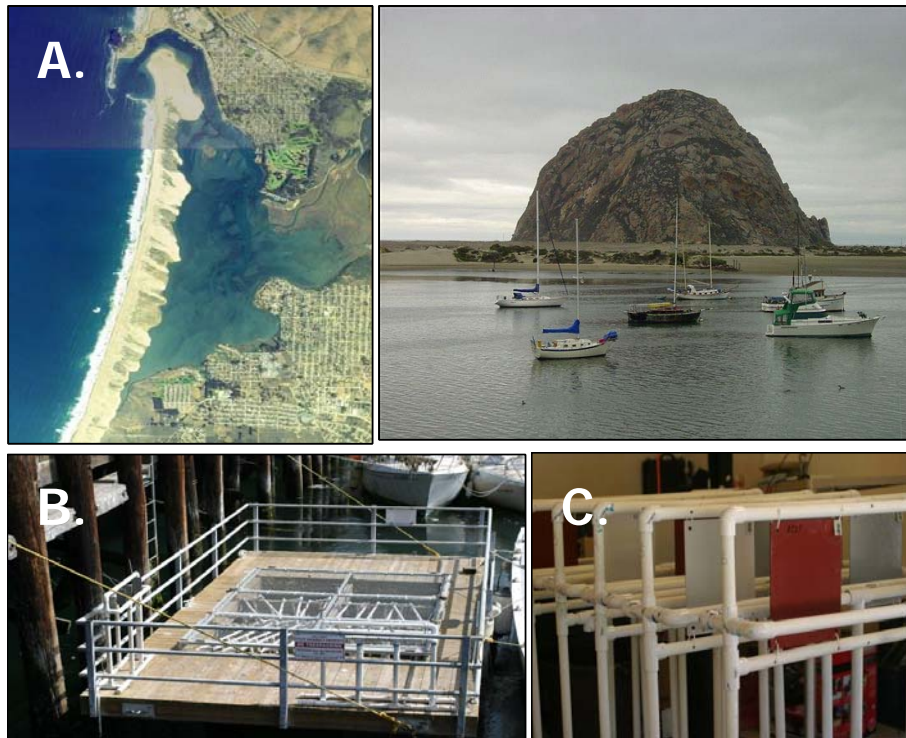
Figure 1. California Polytechnic State University test site at Morro Bay, California. A. Morro Bay. B. Floating dock supporting baskets for panels. C. Mounting of panels in baskets.
