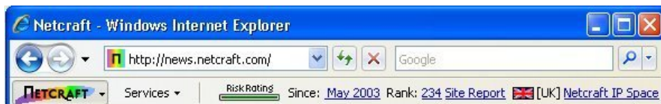
Figure 3.1: Passive warning in Netcraft. Presents information like risk rating of the website, year of registration of the website, popularity of the website among toolbar users, and an image of a flag or a two letter country code where the website is hosted.
