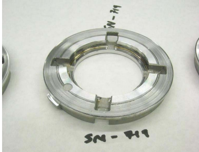
Figure 15 - SN719 Retainer Plate Wear
