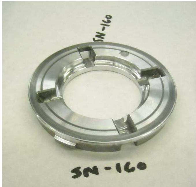
Figure 20 - SN160 Retainer Plate Wear
