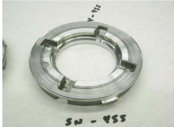
Figure 11 - SN455 Retainer Plate Wear
