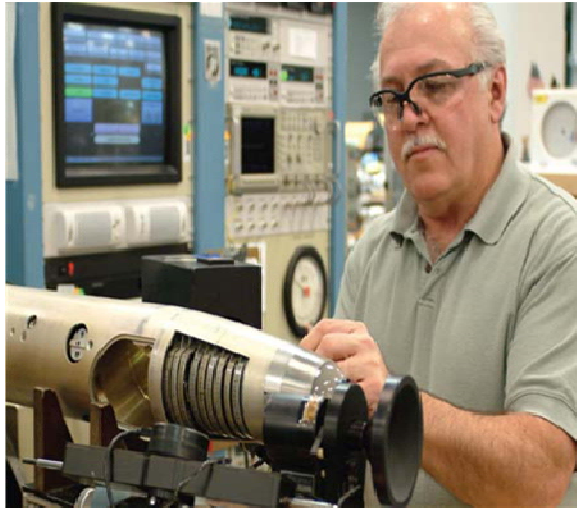
Figure 7. This picture shows an Electronics Technician repairing a Guidance and Control Section (GCS) of the Sidewinder Missile [From (Tobyhanna Army Depot, 2007)].
