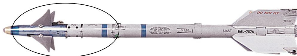
Figure 1. AIM-9 Sidewinder Missile with Guidance and Control Section (GCS) circled [After (U.S. Air Force, 2007)].
