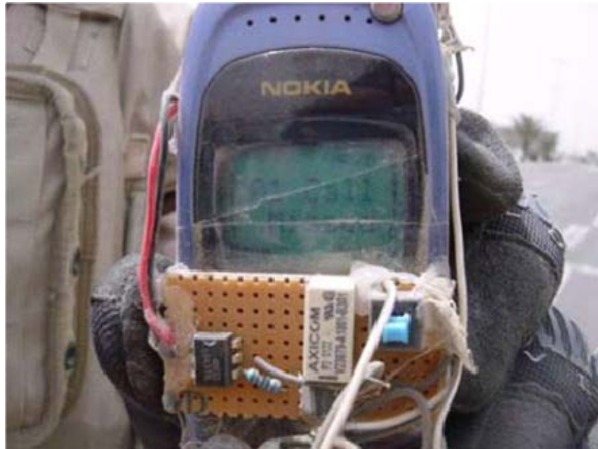
Figure 1. A soldier holds a RCIED using a cell phone as the triggering device
