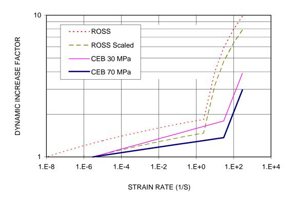
Figure 1. Ross scaled versus CEB for concrete in tension.
