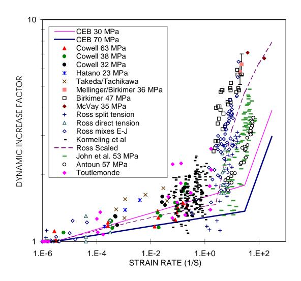
Figure 2. Ross scaled and CEB versus test data.
