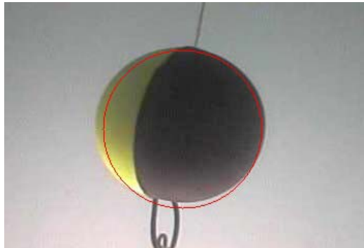
Figure AORD-17. Result of video processing: the circle extraction.
