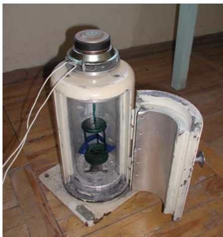
Figure 17: The experimental lead chamber with IS frequency vibration stand and ELF EMF–generating coil constructed in it
