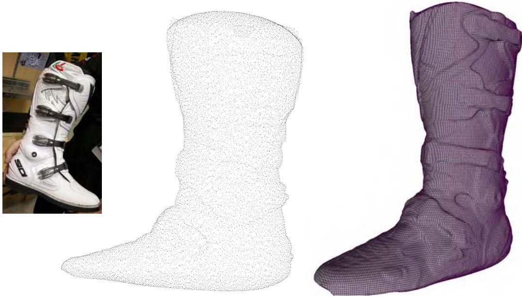
Figure 5. Left image is photograph of motocross boot. Middle image is rendering of 10% of the approximately one million data points scanned from a physical boot. Right image is a rendering of isosurface extracted from implicit model.
