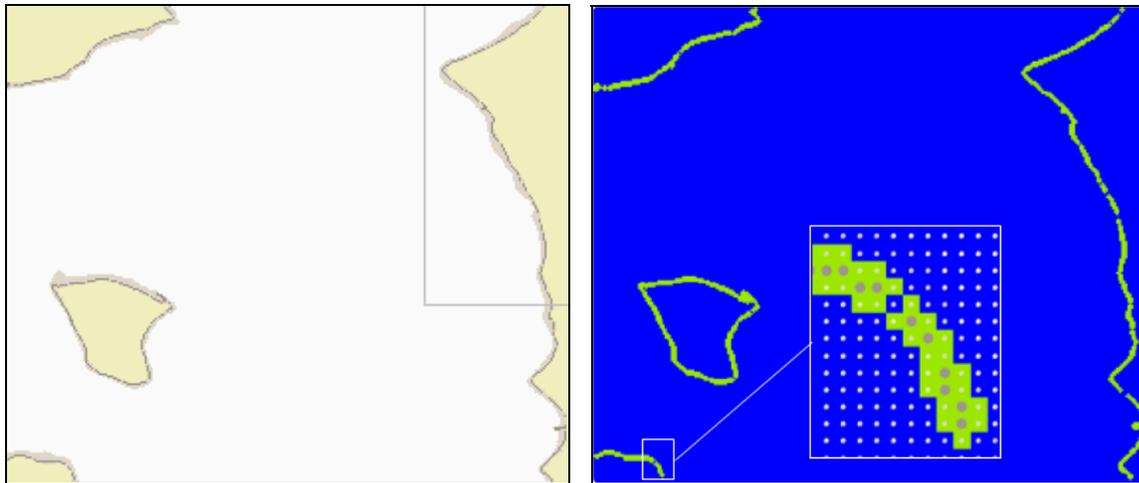
Figure 2. Example of clustering by geospatial location and color: all pixels within a predetermined distance in geospatial ( $x=1$ ,  $y=1$ ) and color ( $z=9$ ) space of the shoreline pixels (brown pixels in the original image, left) are clustered together. The resulting clusters are shown in green, right. The zoomed-in section shows a detail of the pixels being clustered.
