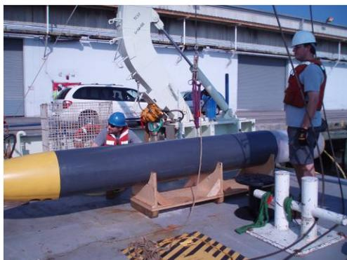
Figure 6: Snag resistant depressor with fairing.
