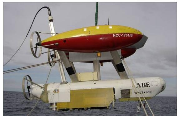
Figure 5: ABE Vehicle showing cable spool at bottom left and mast
