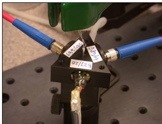
Figure 7 - Reduced volume flow-cell designed for ratiometric measurement
