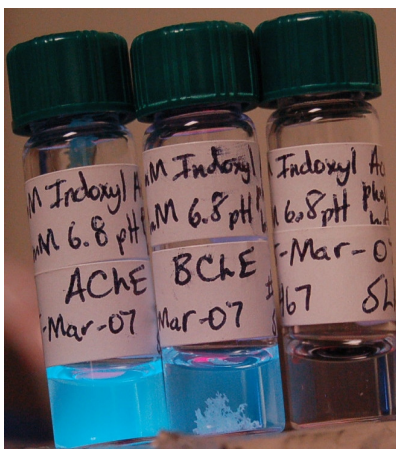
Figure 4 - Fluorescence from a vial of indoxyl acetate after with AChE sponge (left), BChE sponge (middle), and no sponge (right),
