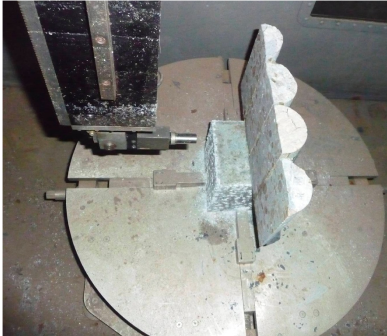
Figure 15. Specimen on Turntable with Scanning Arm and Transmitting / Receiving Transducer (Tank is Dry).
