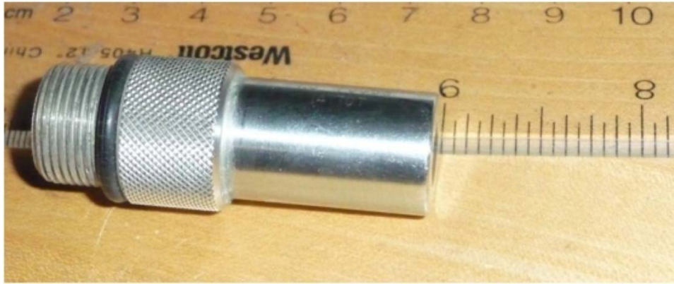
Figure 13. 15 MHz Ultrasonic Transducer with a 1-inch Focal Distance used for Reflection Imaging.
