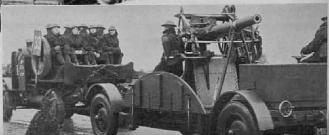
This is a British 3-inch AA gun on a 4-wheeled mount.
