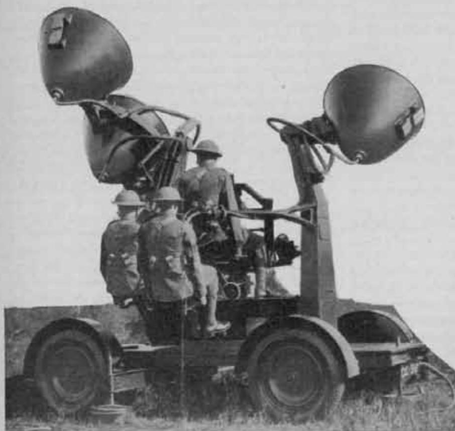
Left: Latest type British sound locator. Note the three-horn arrangement. Right: Latest type British director.
