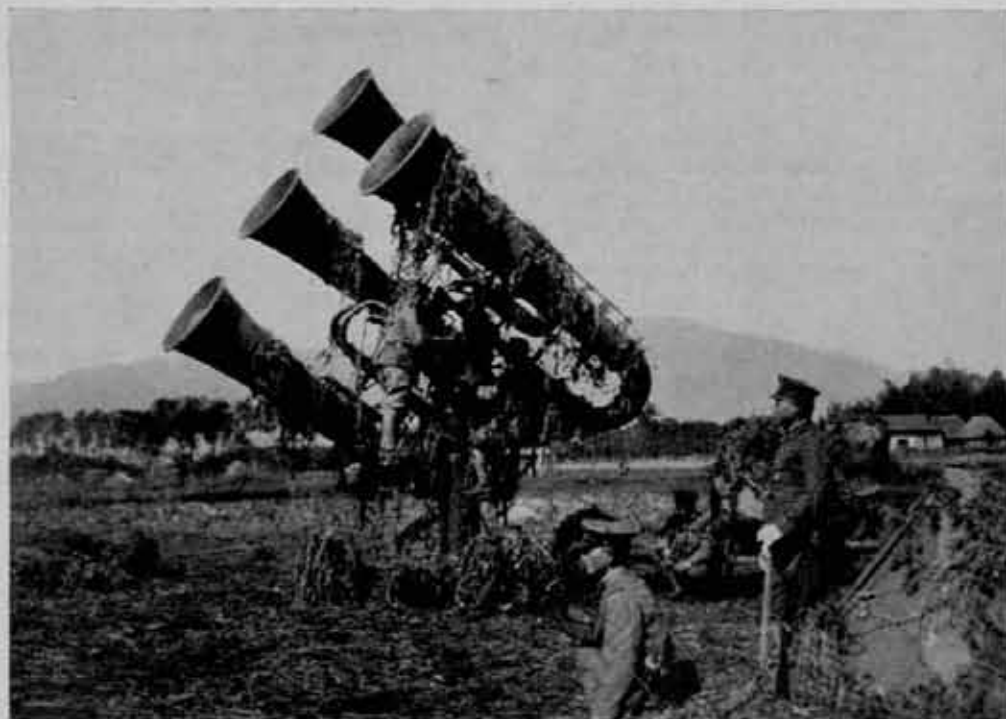
Latest type Japanese anti-aircraft sound locator.
