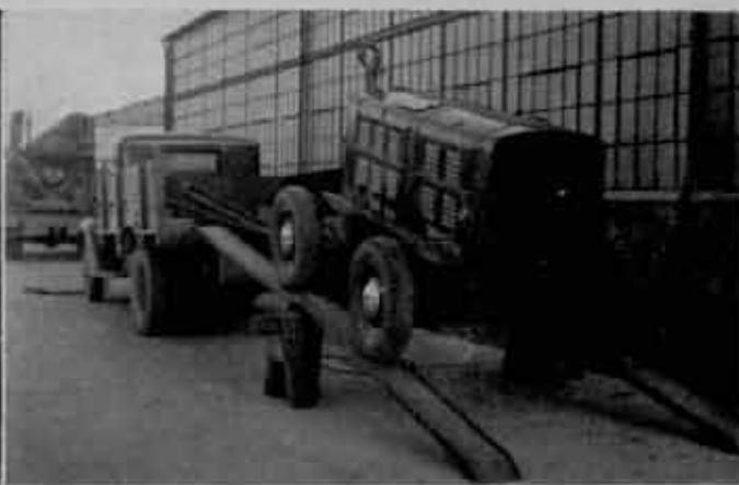
Right—Loading power plant into standard cargo truck.
