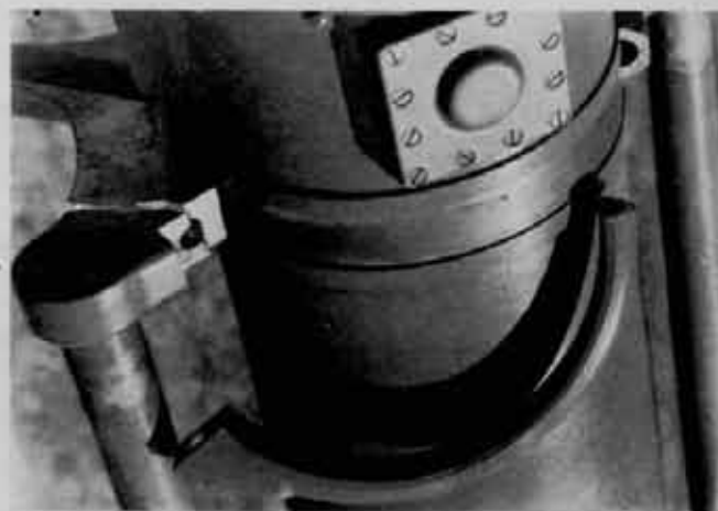
Height Finder Tube, showing broken bracket for porter bars.
