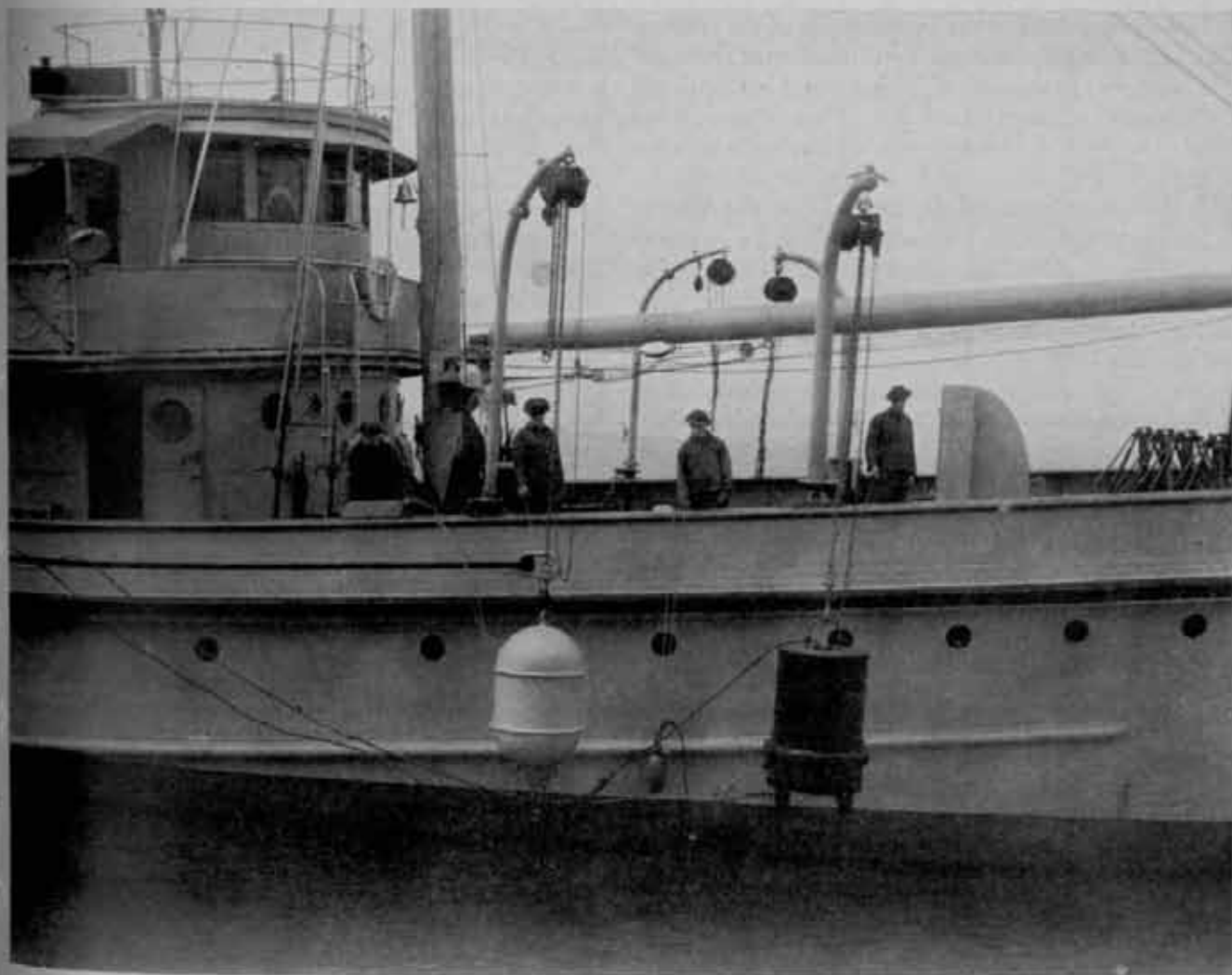
Mine, anchor, and marking buoy go over the side
