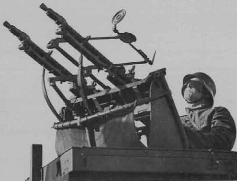
This is a German heavy anti-aircraft machine gun on a dual mount. The weapon is mounted on a trailer body that can be horse or motor drawn.
