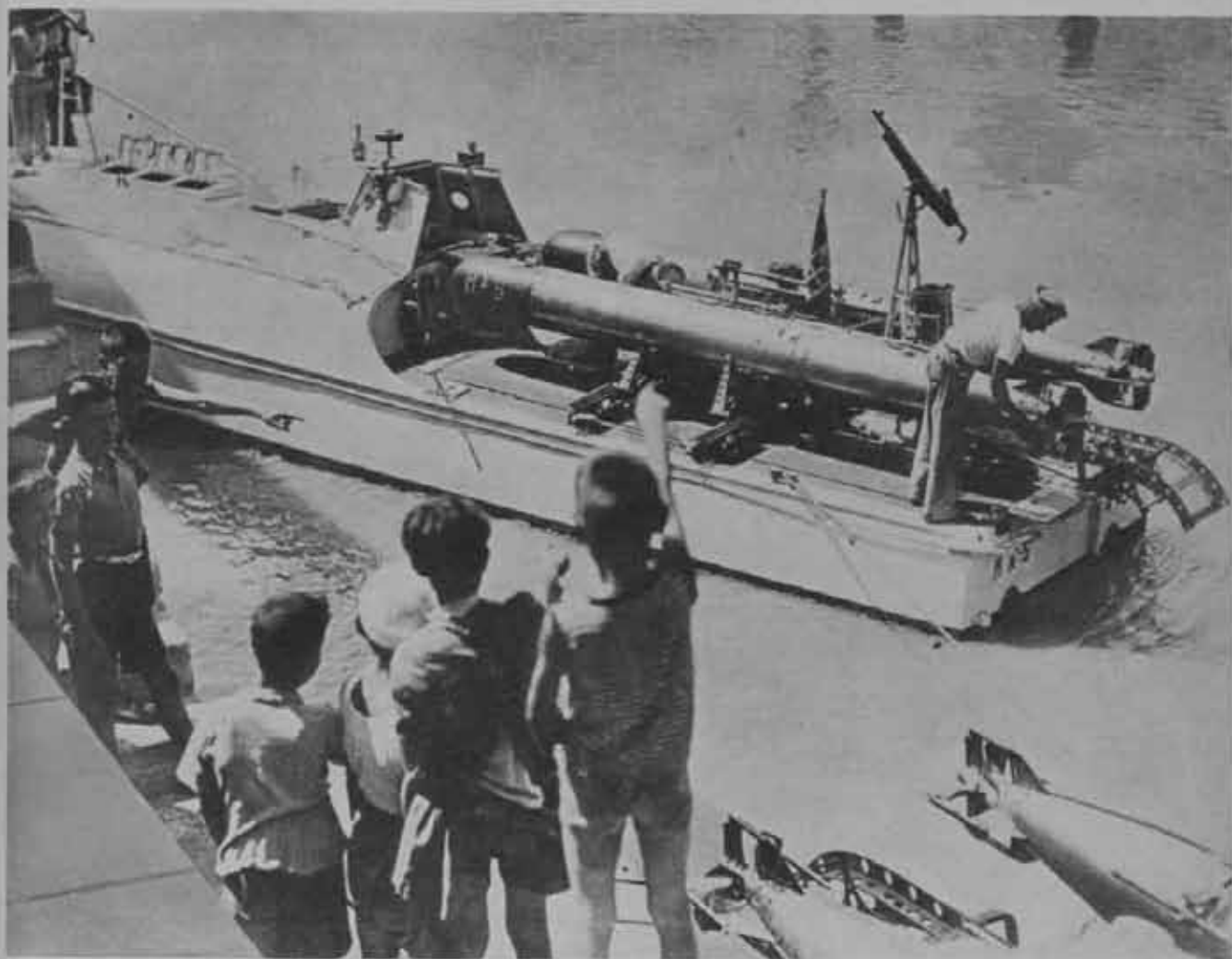
This Italian motor torpedo boat is admirably suited for action in quiet and narrow waters. Its speed of 45 knots makes it excellent for reconnaissance, shadowing, and attack.
