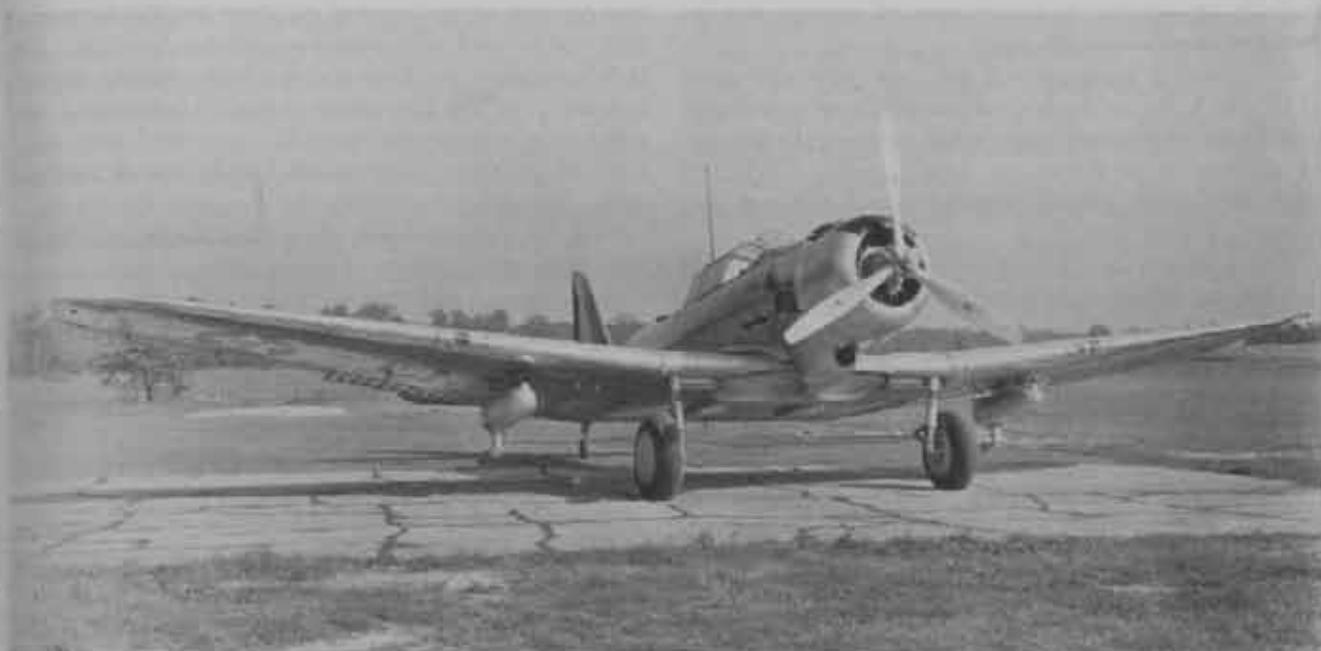
Figure 1: Attack airplane (A-17) (With chemical spray tanks).
