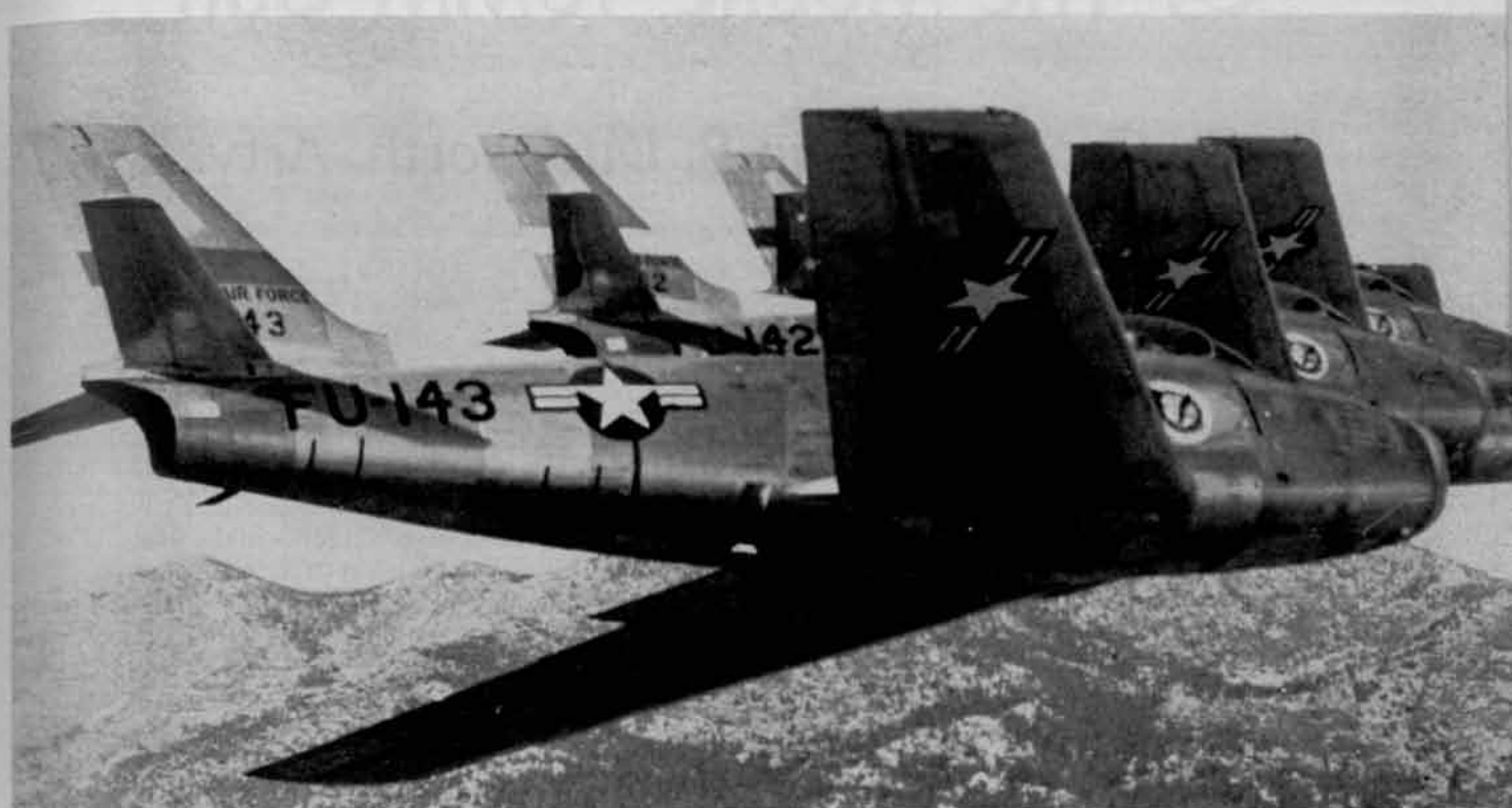
A formation of four North American F-86 "Sabres." Their speed is well over 650 mph with a ceiling of over 45,000 feet. These jet fighters were recently credited with destroying attacking jet planes over North Korea.
