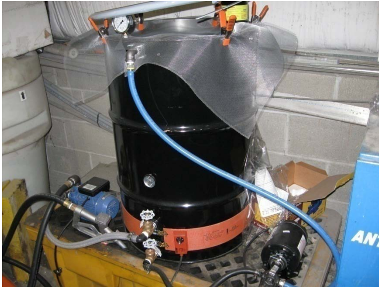
Figure 8: High Cost Fryer to Fuel WVO to SVO System (Photo by Harvey S. Gaber)
