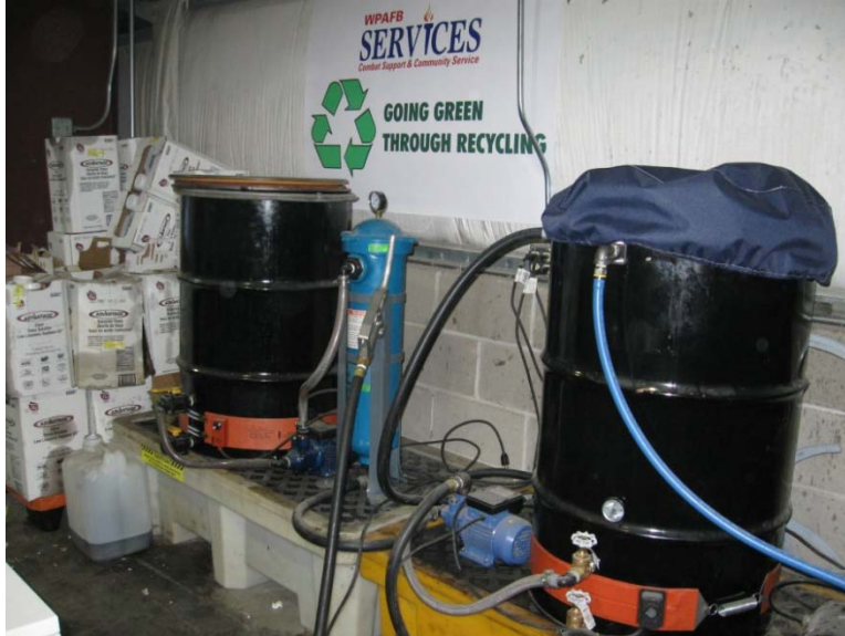
Figure 9: Complete WVO to SVO Processing System (Photo by Harvey S. Gaber)
