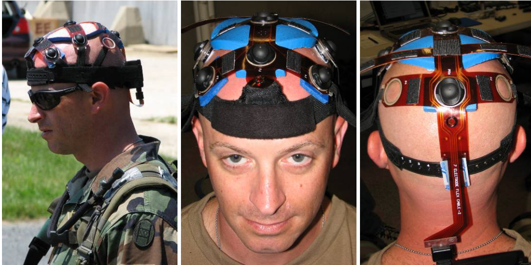
Figure 2. ABM's wireless EEG sensor headset.
