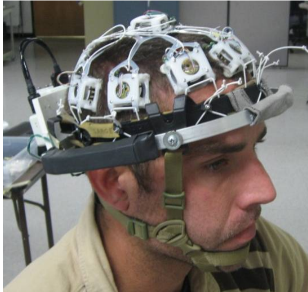
Figure 12. QUASAR's wireless EEG sensor headset.
