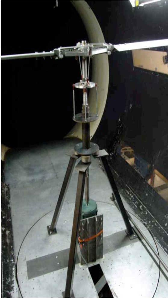
Figure 0: Dynamic Stall rig assembly in the test section of the John J. Harper wind tunnel
