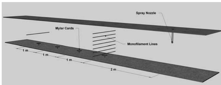
FIG. 2—Deposition and flux sampling locations.
