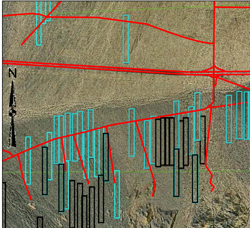
Figure 8. Example in southern California of the intersection of roads (red lines) with OLSs (blue rectangles). OLSs not intersected by roads are outlined in black. The OLSs are 930 m long and 90 m wide.
