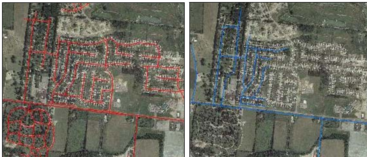
Figure 6. Tele Atlas primary and secondary road vectors, in red, overlying a DOQ (left) and USGS DLG roads, in blue, overlying the same DOQ (right). Secondary roads are not as completely represented on the USGS product.
