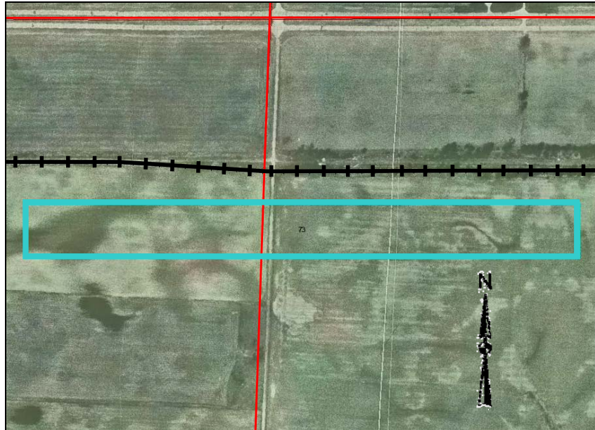
Figure 10. Intersection of a road (red lines) with an OLS (light blue rectangle) in southern Indiana. The hatched black line is a railroad. The OLS is 930 m long and 90 m wide.
