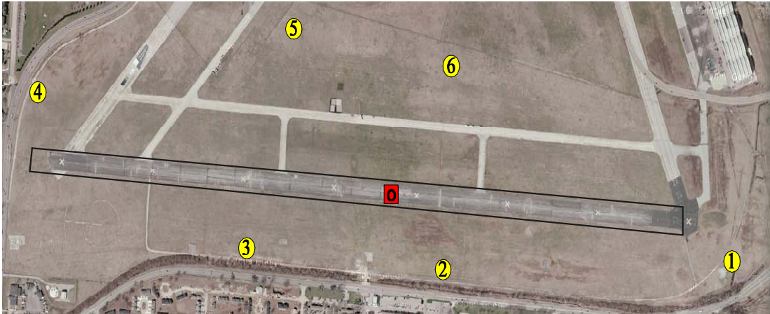
Figure 3.5: Pseudolite Tower Positions Relative to the Runway used for the Field Test.
