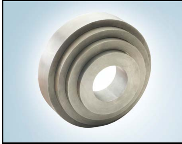
Figure 4. Exploded view of Anviloy rings capable of producing bearing loads from approximately 44 to 176 N. (Steel housing for 35 mm bearing not shown).
