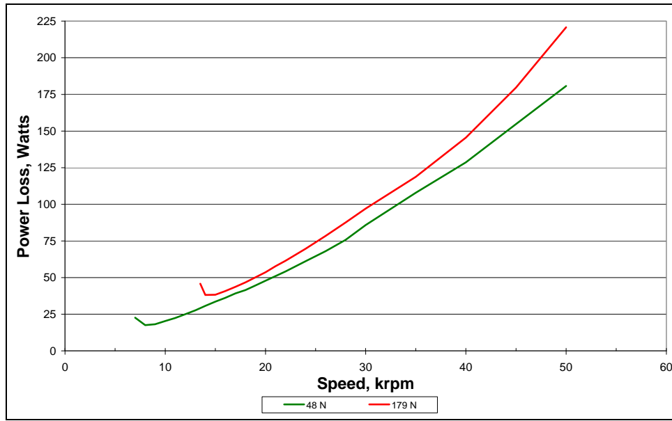
Figure 9. A 2-D performance map for the 51-mm diameter, 51-mm long foil bearing.
