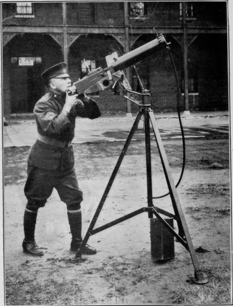
FIG. 1. .30 CALIBER BROWNING MACHINE GUN, MODEL 1917, MOUNTED ON ANTI-AIRCRAFT TRIPOD, MODEL 1918
