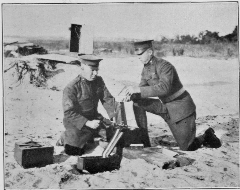
FIG. 7. BELT FILLING STATION, SHOWING NO. 5 AND NO. 6 OPERATING BELT FILLING MACHINE
