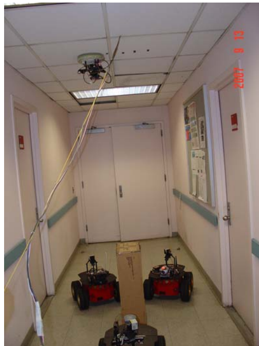
Fig. 1 Experimental settings for 3D map construction using 3 ground robots and a City-Climber robot
