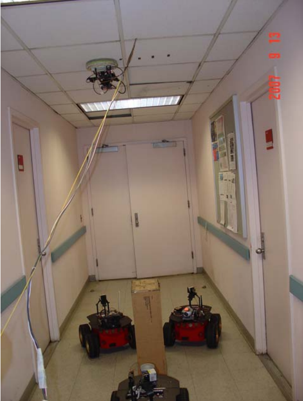
Fig. 7 Experimental settings for 3D map construction using 3 ground robots and a City-Climber robot
