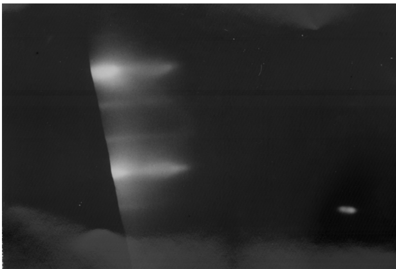
Figure 23. Reflection high energy electron diffraction pattern of GaN:Gd, T_{\text{Gd}} = 1050^\circ\text{C} . The picture shows a 2D/3D pattern with 1\times 3 reconstruction.
