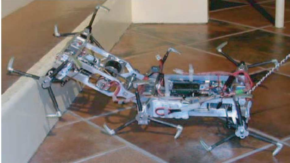
Figure 2.3: WHEGS™ II Rearing Half of Its Body [11].
