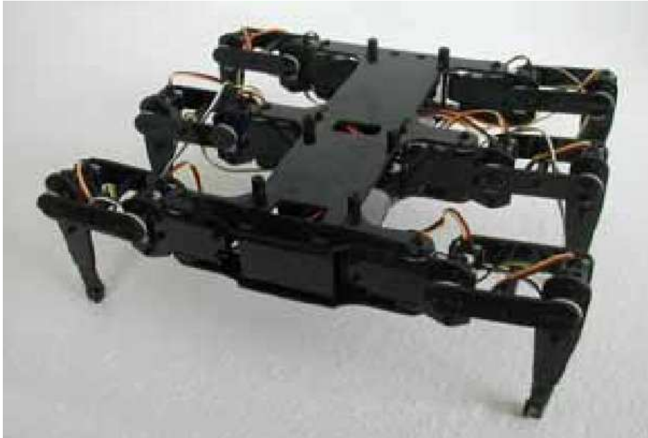
Figure 2.6: Hexapod III Kit Constructed and Wired [18].
